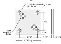
**Construction:** Black oxide finish, two mounting screws furnished.
